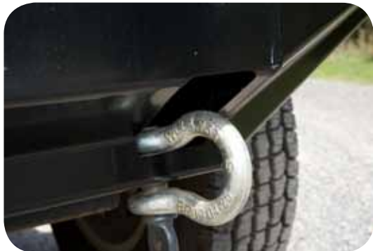
Integrated tow point in Hi-Lift jacking mount allows fitment of 4.75t bow shackle upright
