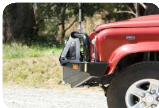
Close fitting design retains maximum approach angle
