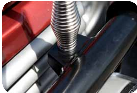
Two CB aerial brackets are mounted on the top tube
